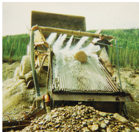
Ted Takacs placer mining operation: loader feeding sluice.
